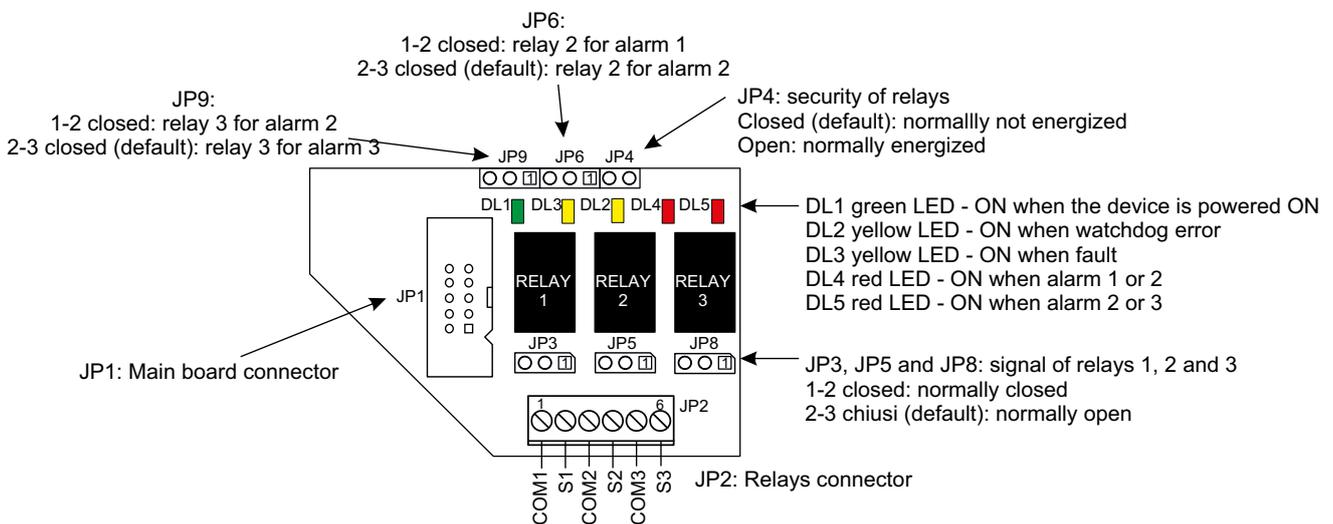
Figure 4) 3 relays board
